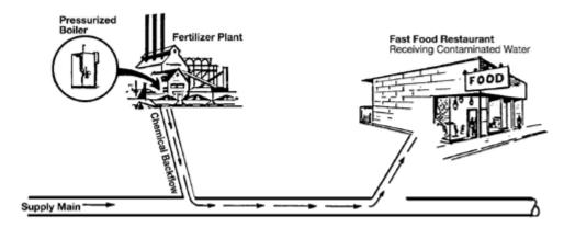
The supply line to the pressurized boiler at the fertilizer plant was leaking, which allowed chemicals in the boiler to backflow into the water main supplying the fast food restaurant next door.
