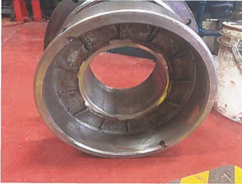
UPPER GENERATOR RADIAL GUIDE BEARING Bottom View
