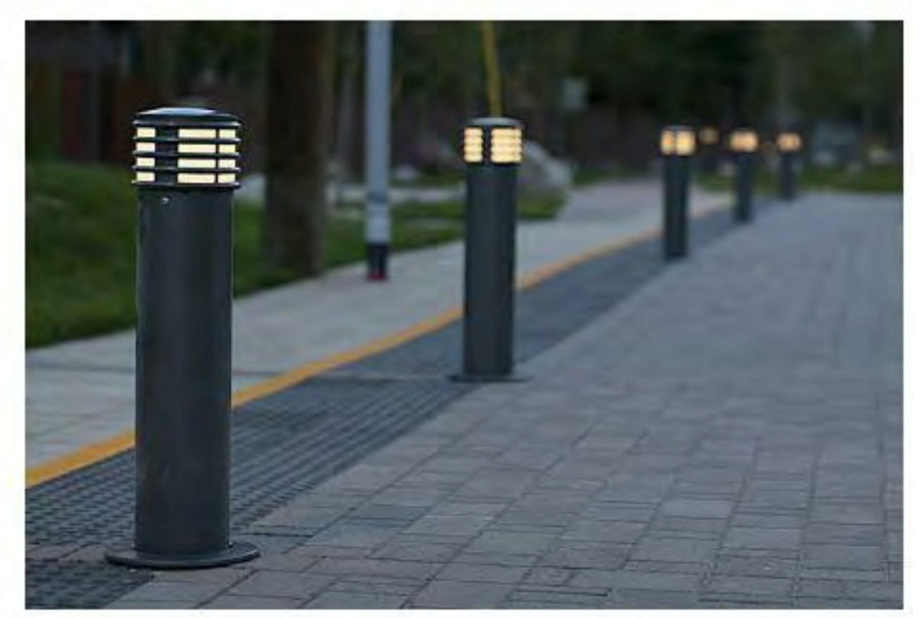
BOLLARD FIXTURE SCHEDULE: *1" 6" NOMINAL DIAMETER METAL BOLLARD. QUANTITIES AS INDICATED ON ELECTRICAL SITE PLAN. FINISH SHALL BE POLYESTER POWDERCOAT, RUST, CHIP AND UV RESISTANT IN BLACK. LOW VOLTAGE LED WITH INTEGRAL DRIVER AND INPUT LINE VOLTAGE SHALL BE 120V, EMBEDDED MOUNTING. LED AND DRIVER SHALL HAVE A MINIMUM 5 YEAR WARRANTY. LANDSCAPE FORMS - ANNAPOLIS BOLLARD
