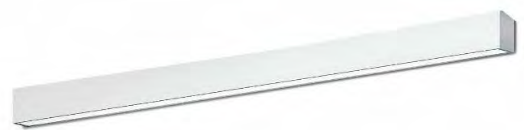
CANOPY FIXTURE SCHEDULE: *1" WALL MOUNTED LINEAR SLOT LED, 2" W NOMINALLY WITH EXTRUDED ALUMINUM HOUSING, SEAMLESS GLARE-FREE FLUSH WHITE OPTIMIZED DIFFUSER. PROVIDE WITH CONTINUOUS RAILS WITH AND >90 CRI, WET LOCATION LISTED. PROVIDE TOTAL LENGTH SHOWN ON PLANS. PROVIDE WITH DRIVER COMPATIBLE WITH DIMMING SYSTEM FOR 0-10V-10% AND 120V OPERATION. PROVIDE CUSTOM COLOR TO MATCH CANOPY STRUCTURE. WALL MOUNTING BRACKET SHALL HAVE SET SCREW FROM BELOW FOR ACCESSIBILITY. PROVIDE GASET BETWEEN ALUMINUM MOUNTING BRACKET AND STEEL STRUCTURE. SELUX- M80 WET LOCATION LED DIRECT SERIES
