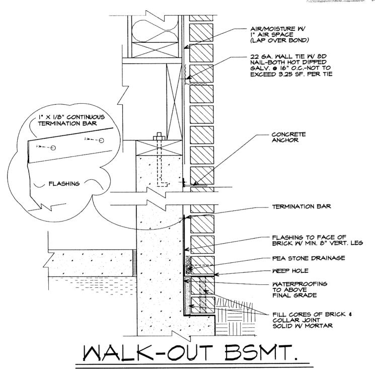
STEP/LAP FLASHING MIN. 8"-12" FORM END DAMS AT END OF RUNS
