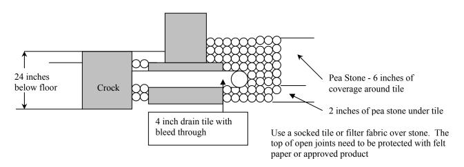
If using a gravel, crushed stone, or other approved material as a drain
